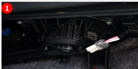
① Remove OEM blower motor connector
