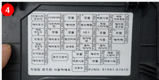
④ Connect ACC depending on the vehicle (optional) / cigar lighter, ACC, power outlet
