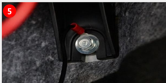
⑤ Connect the ground to the body bolts
